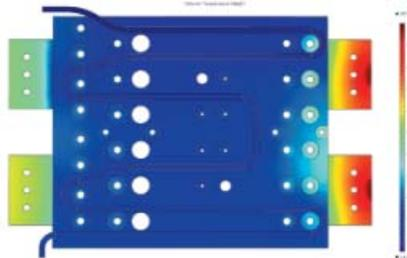
Figure 7: Thermal simulation for a water-cooled busbar
