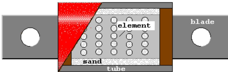
**Fig.2 Construction of a typical current-limiting fuse.**
