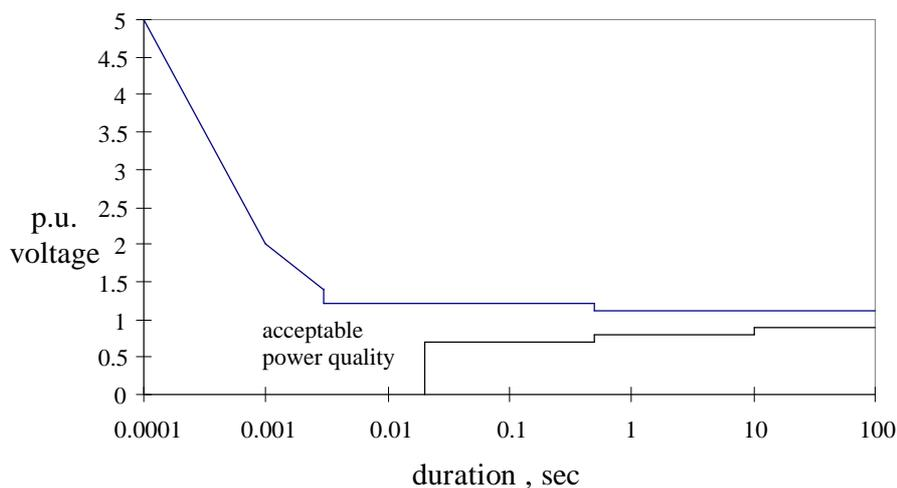
**Fig.1 ITIC (CBEMA) curve.**
