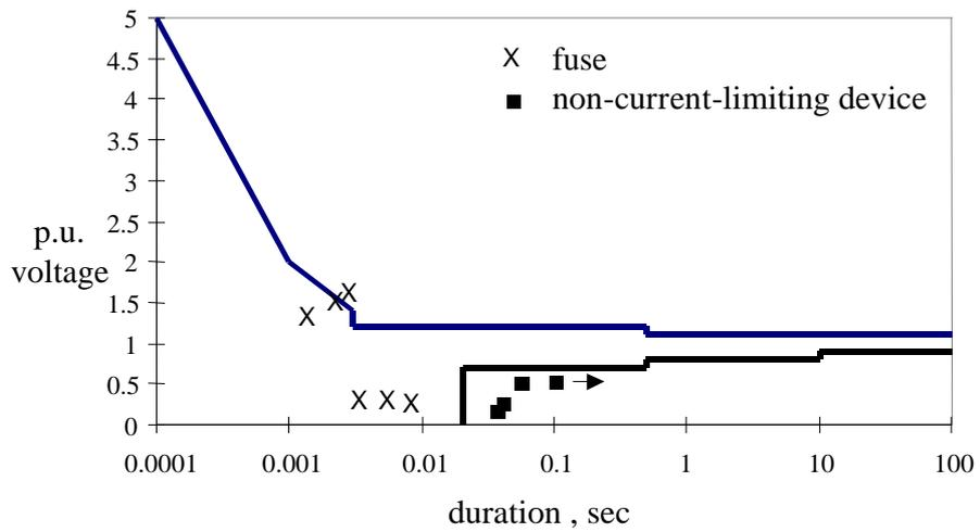
**Fig.7 Voltage sags and peaks in relation to ITIC curve.**
