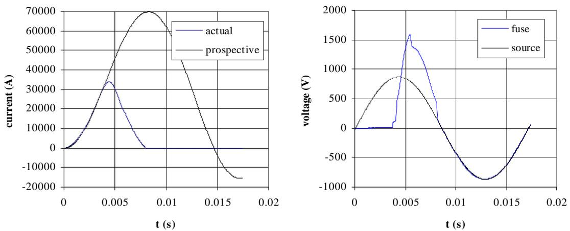
**Fig.3 Waveforms for breaking of an a.c. short-circuit by a current-limiting fuse.**
