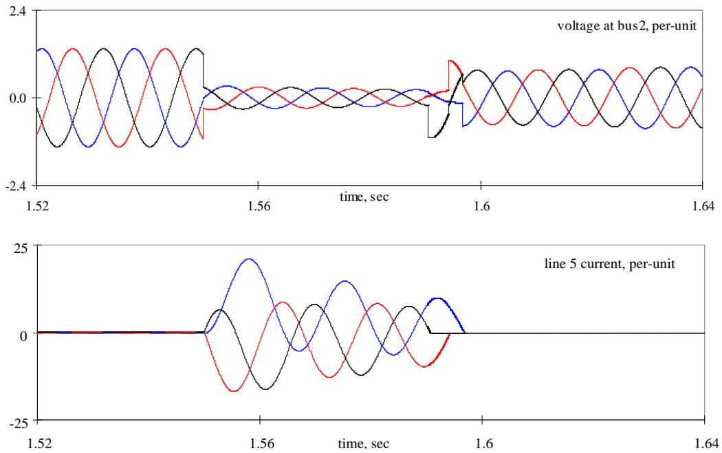
**Fig.6 Transients in system protected by non-current-limiting devices.**
