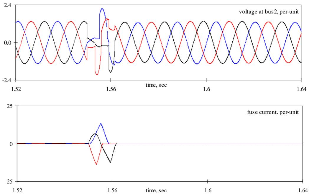
**Fig.5 Transients in system protected by current-limiting fuses.**
