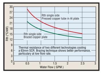
**Fig. 4**. The brazing technique shows better performance than the pressed copper tube in aluminum plate technique, as you can see in this comparison between the two technologies.
