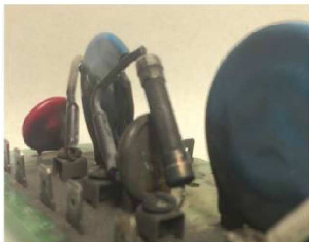
A failed 20mm MOV that was "protected" by a thermal fuse
