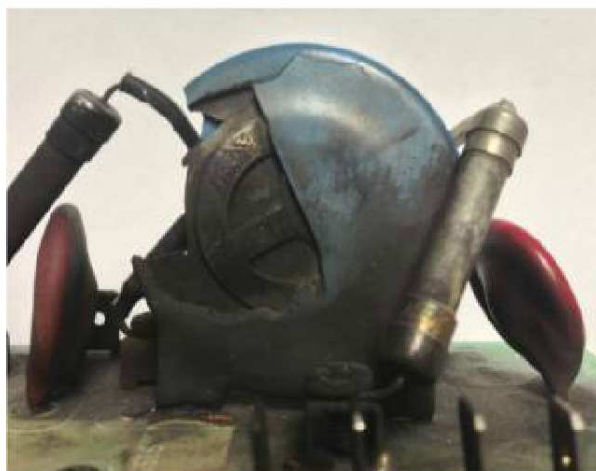
A failed 40mm MOV that was "protected" by a thermal fuse
