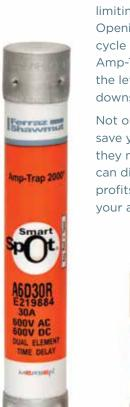
Mersen's Amp-Trap 2000 currentlimiting fuses do more than that. Opening in less than one-quarter cycle at fault currents up to 300kA, Amp-Trap 2000 fuses minimize the let-thru current that flows downstream.
