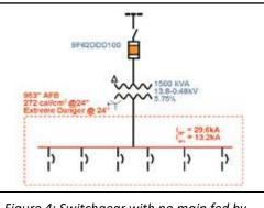
Figure 4: Switchgear with no main fed by 1500KVA Transformer. Short circuit protection for switchgear bus is provided by primary fuse.
