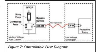
The example shown in Figure 8a demonstrates how to model the two fuse elements and Bypass switch of the Controllable Fuse in power system analysis software with conventional elements. In this diagram the 50P unit of the relay, wired to CTs on the secondary of the transformer, is shown connected to the Bypass Switch of the Controllable Fuse. When modeled in this manner, the time current curve of the Main Fuse would be used to assess the level of protection on the primary of the transformer and
