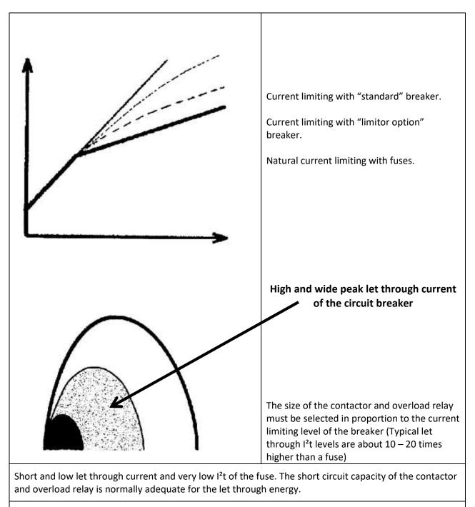
Current limiting fuses clear short-circuit fault in less than a half-cycle, improving the "power quality" in the system.
