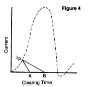
The fuse that clears in time A will provide better component protection than will the fuse that clears in time B.
