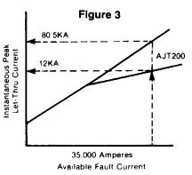
Figure 3 illustrates the use of the peak let-thru current graph. Assume that a 200 ampere Class J fuse (#AJT200) is to be applied where the available fault current is 35,000 amperes RMS. The graph shows that with 35,000 amperes RMS available, the peak available current is 80,500 amperes (35,000 x 2.3) and that the fuse will limit the peak let-thru current to 12,000 amperes.
