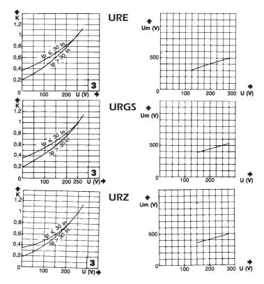
$<sup>^{*}</sup>$  The mean curves show the variation of the total clearing time ( $^{12}t_{t}$ ) and the total clearing duration  $t_{t}$  as a function of operating voltage U
